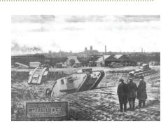
**Tank Fact:** Tanks had a crew of eight men, four men were needed for the driving operations. Steering involved engaging different gears on each side of the tank in order to swing it to one side.
